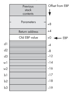
Figure 8-10: Aligned variables in an activation record
