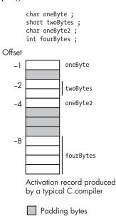
Figure 8-9: Padding bytes in an activation record
