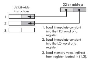
Figure 8-2: RISC CPU access of an absolute address
