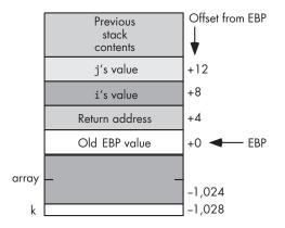
Figure 8-6: Activation record for BigLocals function
