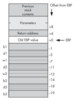
Figure 8-11: Unaligned variables in an activation record
